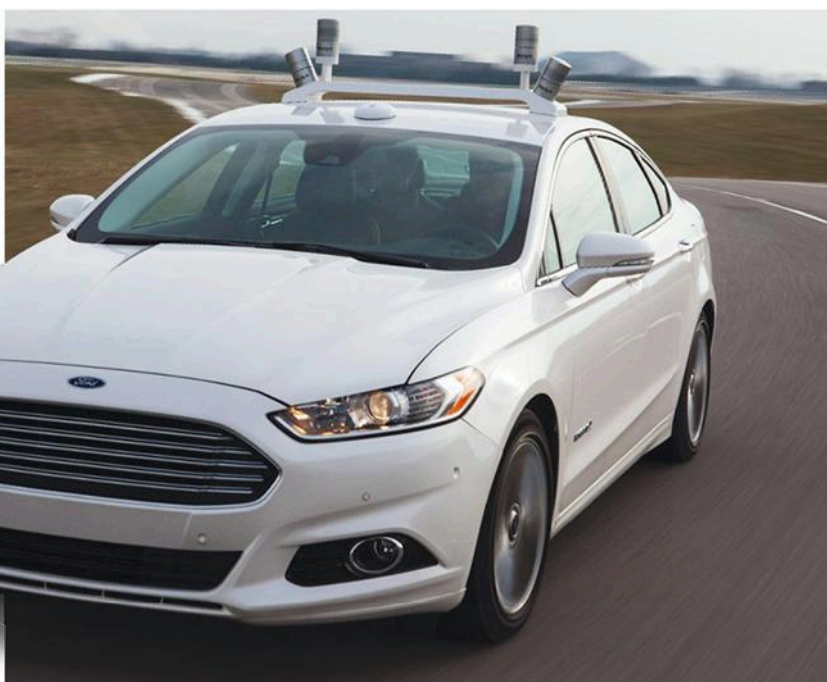
1. Ford's experimental Fusion Hybrid has the obvious LIDAR on the roof, but there are a host of other sensors and support hidden throughout the car.
