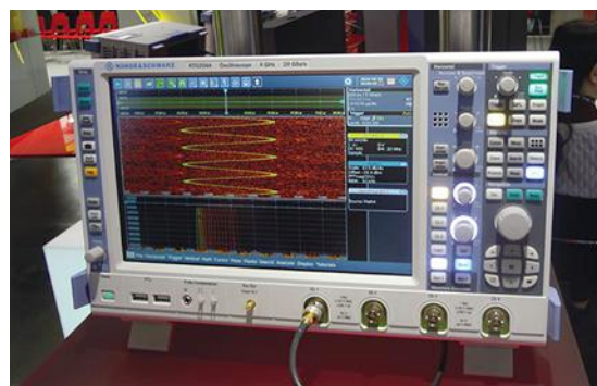
2. Rohde & Schwarz's RTO2000 oscilloscope can use zone triggering within the frequency domain.
