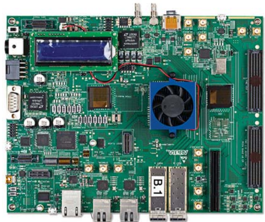
Figure 2. Arria 10 SoC Development Kit Board
