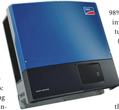
3. The Sunny Tripower TL-US delivers advanced smart-inverter features, including active power curtailment; adjustable power factor and reactive power supply; frequency and voltage ride-through; and soft-start reconnection ramp controls. (Courtesy of SMA)
